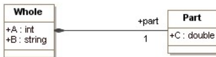
Figure 1.3: Example illustrating composition association: the definition of one class of objects employing another class of objects in a part-whole relationship. In this particular example, an instance of a Whole class object must contain exactly one instance of a Part class object, and the symbol referring to the Part class object is part. In XML, this symbol becomes the name of a subelement and the content of the subelement follows the definition of Part.
